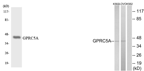
Western blot analysis of the lysates from K562 cells using GPRC5A antibody.
