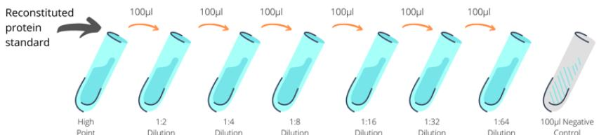
**Two-fold dilution series:** Each microtiter starts with 100µl diluent. 100µl is carried over from the reconstituted protein standard, thoroughly mixed and then 100µl is transferred to the next. The process is repeated in each microtiter in the sequence. No treatment is carried out on the negative control, which should hold 100µl of diluent.
