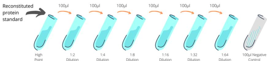
**Two-fold dilution series:** Each microtiter starts with 100 $\mu$ l diluent. 100 $\mu$ l is carried over from the reconstituted protein standard, thoroughly mixed and then 100 $\mu$ l is transferred to the next. The process is repeated in each microtiter in the sequence. No treatment is carried out on the negative control, which should hold 100 $\mu$ l of diluent.
